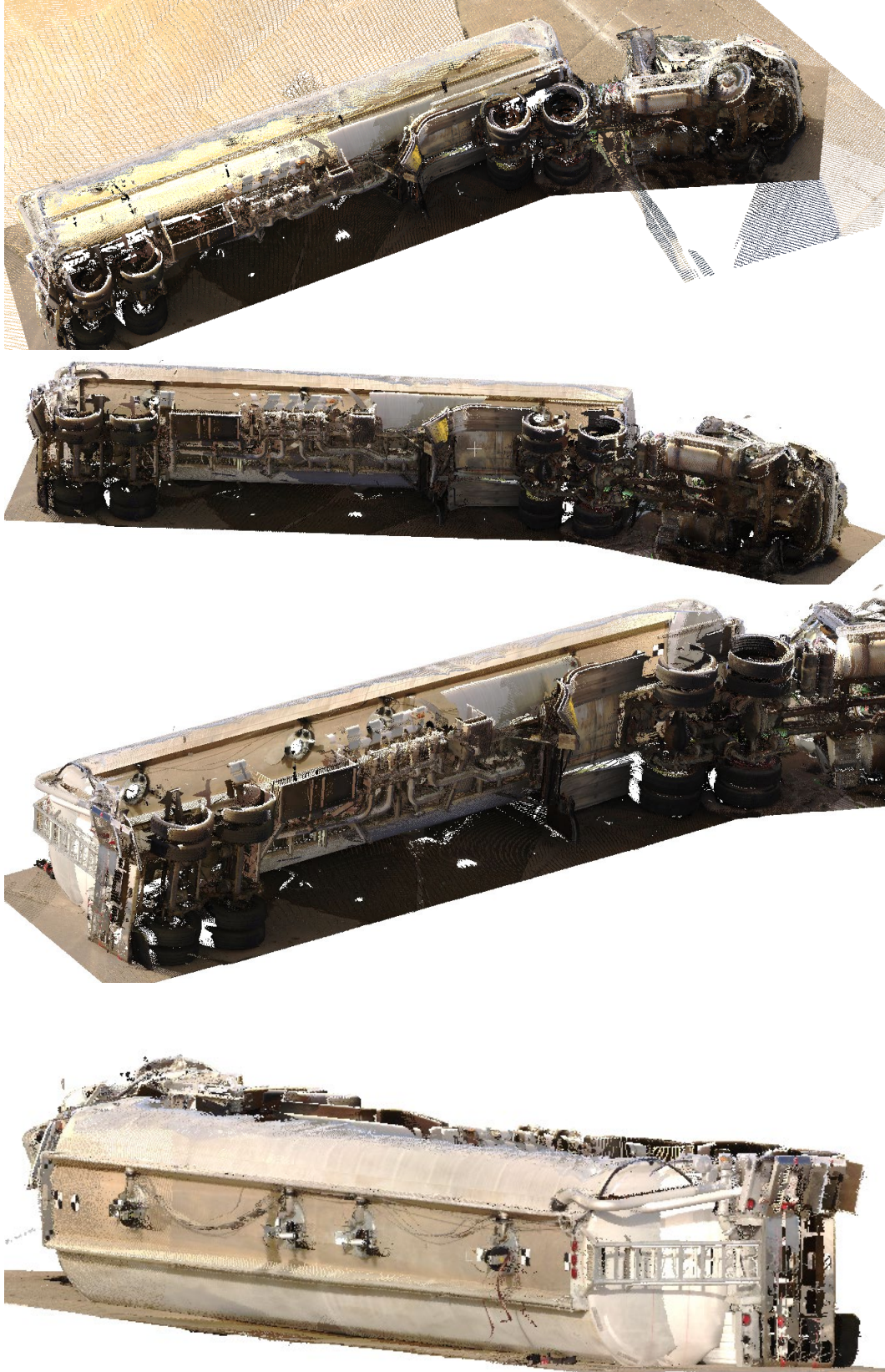
Figure 6.31 Vehicle Scan Results, Tanker Damage, Test No. MTL6-1
