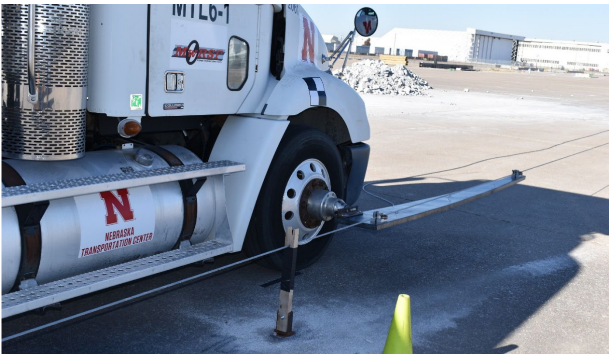
Figure 5.2 Test Vehicle Guidance System, Test No. MTL6-1
