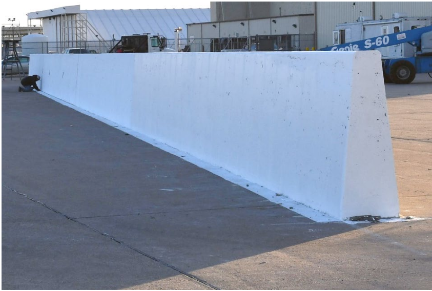
Figure 3.14 MwRSF Optimized TL-6 Single-Slope Barrier Installation, Test No. MTL6-1
