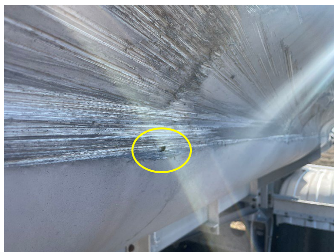
Figure 6.26 Pinhole Damage in Trailer After Being Uprighted, Test No. MTL6-1
