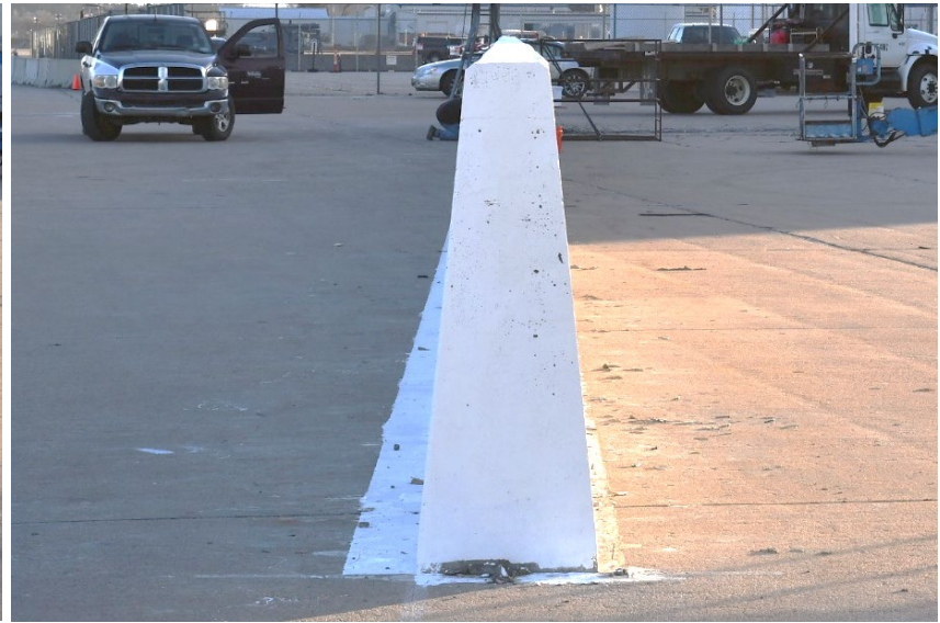
Figure 3.14 MwRSF Optimized TL-6 Single-Slope Barrier Installation, Test No. MTL6-1
