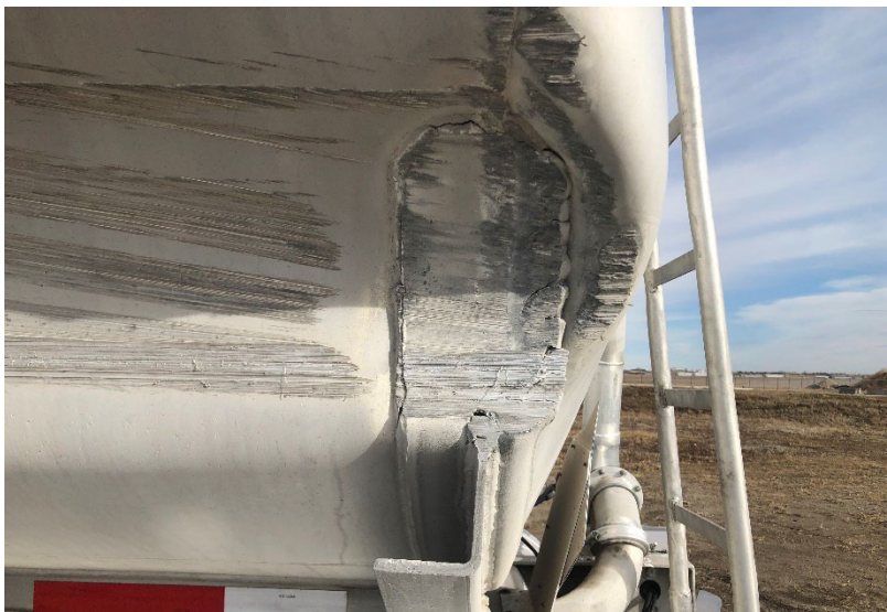
Figure 6.27 Trailer Damage on Impact Side After Being Uprighted, Test No. MTL6-1
