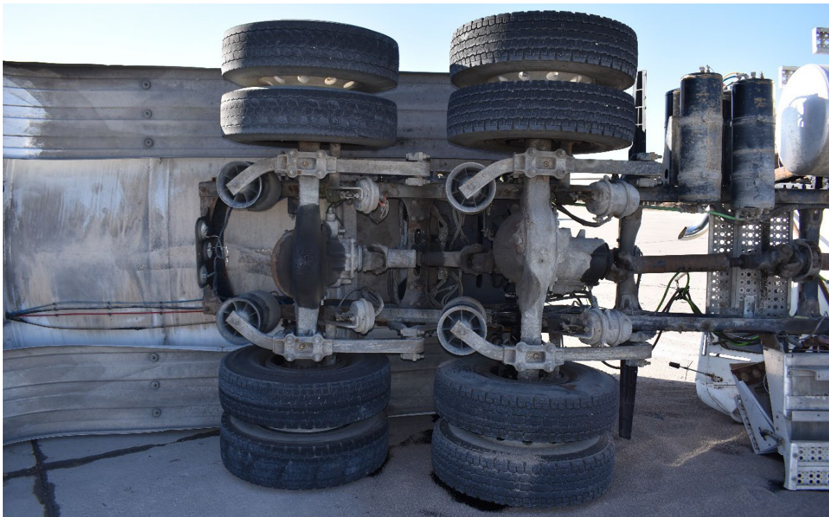
Figure 6.21 Tractor Suspension Damage, Test No. MTL6-1 101
