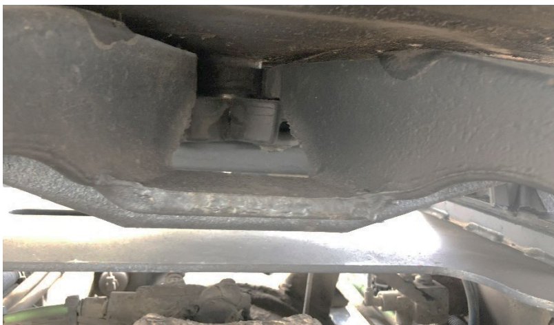
Figure 6.30 Fifth Wheel Damage, Test No. MTL6-1
