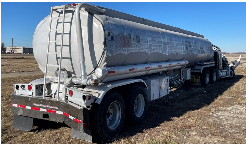
Figure 6.25 Trailer Damage After Uprighting, Test No. MTL6-1
