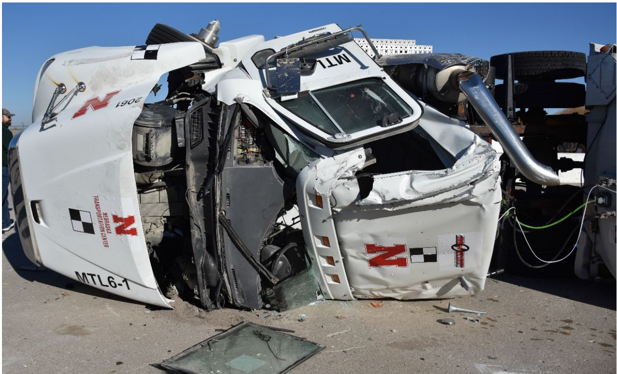
Figure 6.18 Tractor Damage, Test No. MTL6-1
