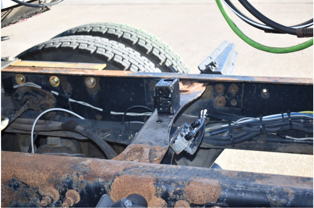
Figure 5.21 Fifth Wheel Camera Mounting Details, Test No. MTL6-1
