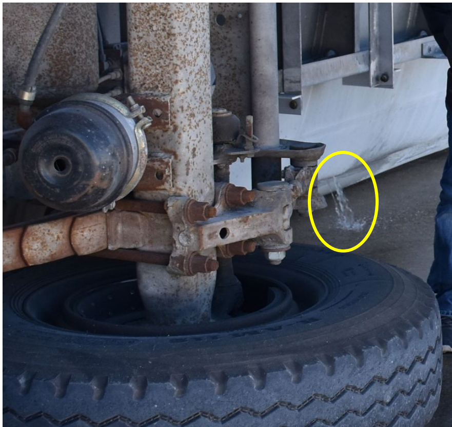
Figure 6.24 Locations of Trailer Leaks, Test No. MTL6-1
