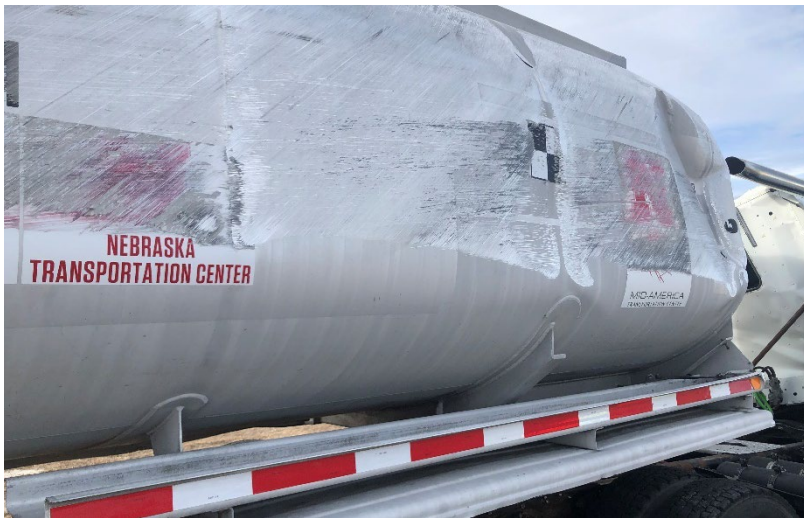
Figure 6.28 Trailer Damage on Non-Impact Side After Being Uprighted, Test No. MTL6-1
