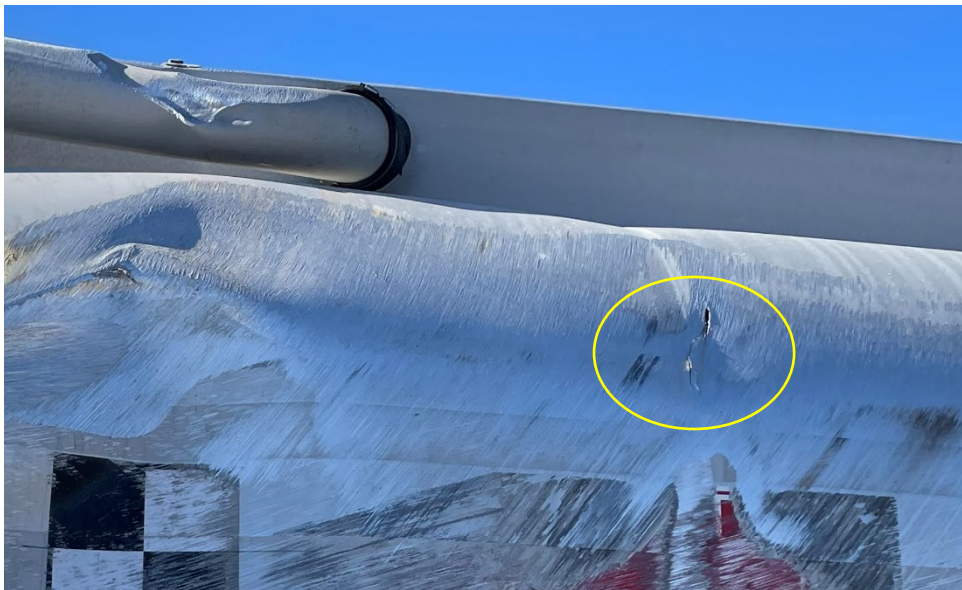
Figure 6.29 Tears in Trailer Jacket on Non-Impact Side, Test No. MTL6-1 109
